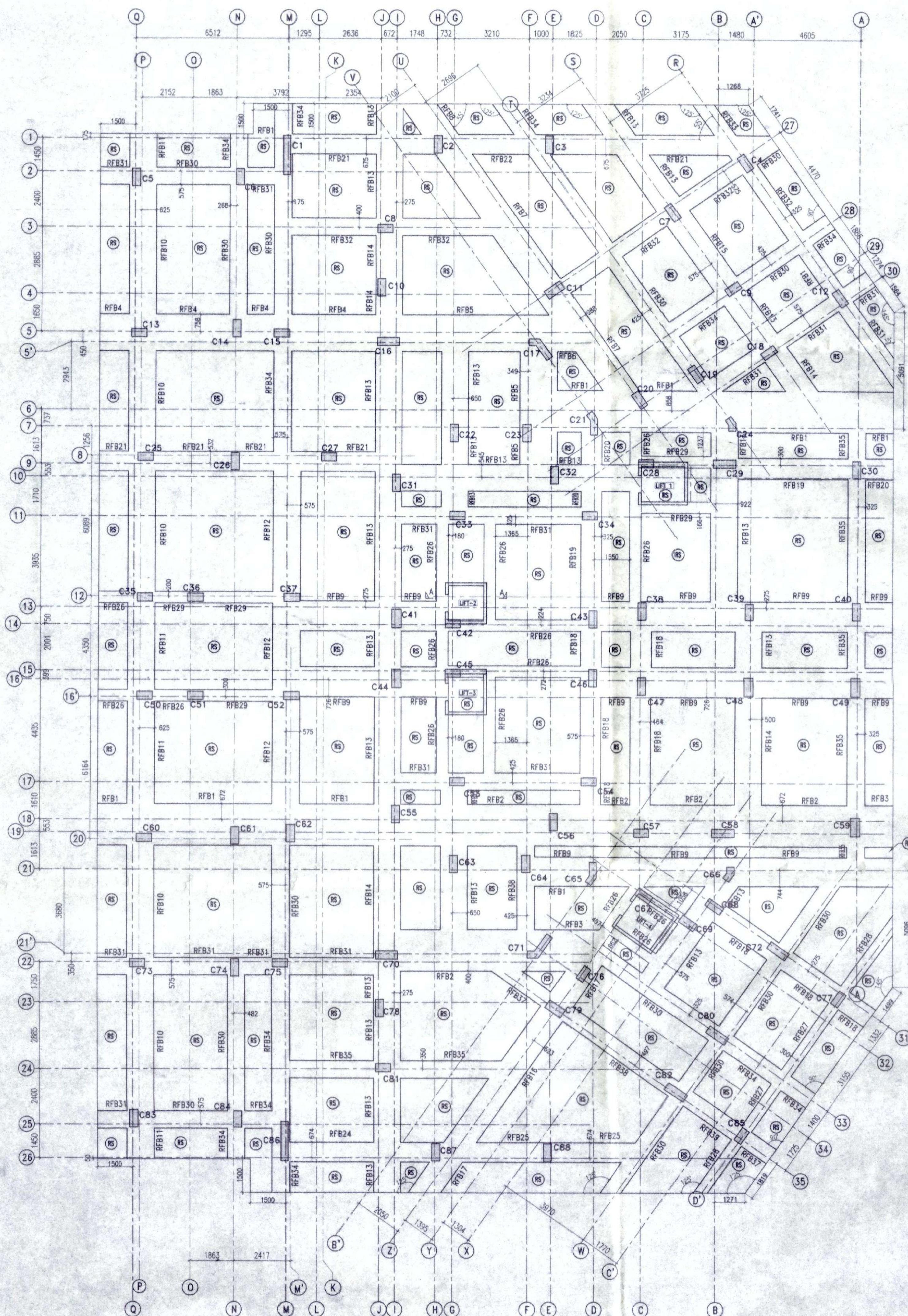
FOUNDATION LAYOUT PLAN RS MARKED SLABS 75mm THK. SCALE: 1:100
